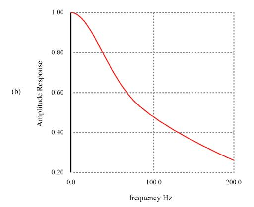
Use 3-dB measure to appropriate estimate the cutoff frequency and the passband width (bandwidth) of the following two low pass filters, represented in dB (or log) and linear scales.
